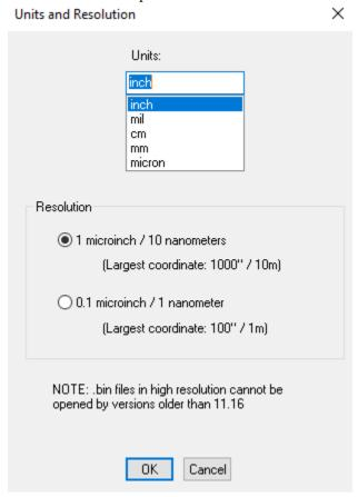
Note that for PCB applications, the "1 microinch" resolution is more than adequate. This was the resolution of previous versions of the software. The new "1 nanometer" resolution is needed when processing chip CAD data.
