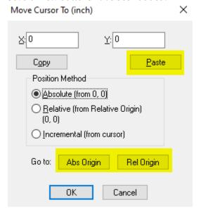
The "Paste" button will paste the text currently in the Windows clipboard into the X/Y fields.
