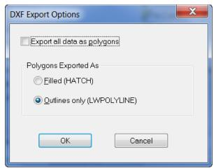
If "Export all data as polygons is checked, then all the data (traces, pads etc.) will be converted internally to polygons and then exported as polygons. This usually results in smaller data files, but they may be harder to edit in AutoCad.
