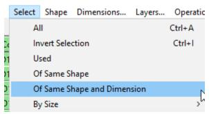
This can be used to select all D Codes that have the same shape type and dimensions, independent of orientation.
