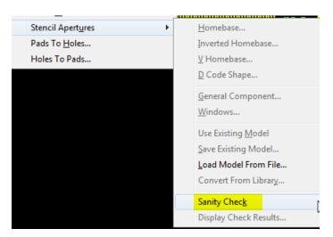
One first needs to make visible only two layers: the pads layer and the stencils layer. The check is done comparing the two layers. Elements are flagged which are out of place, like below:
