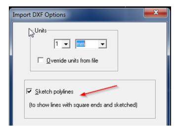
In most cases, when the lines correspond to circuit traces, this option should be left unchecked.
