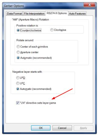
When the "LN" option is checked, the string that appears in the "LN" directive (Layer Name) in Gerber Extended files will set the name of the layer in the CAM software.
