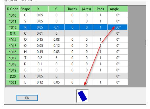
When saving a .bin file, rotated D Codes are converted to custom (M) shapes, to make the output backward compatible with previous versions of the CAM software. When opening these files in the current
