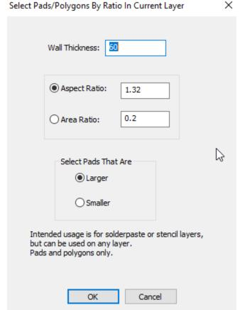
Computation of ratio is based on thickness and the bounding box of each element.
