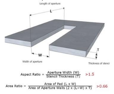
For "Surface Area Ratio" the formula is based on the exact shape of the aperture: area of aperture walls divided by the area of the aperture.
