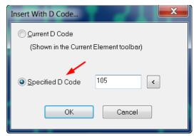
This is useful when during insert operations the current D Code can change (due to aligning or selection) but the user wants to insert using a specified D Code.
