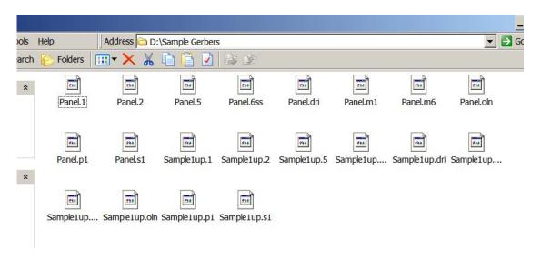
The "Sample1up.\*" files are the originals and the "Panel.\*" files are the panelized Gerber data.
