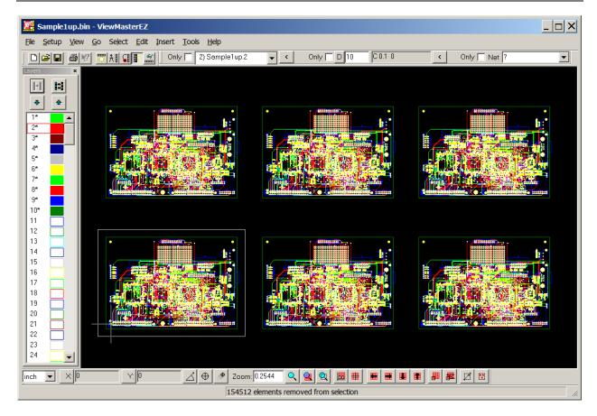
The data is step and repeated as desired. We are now ready to export the data to generate the files to be sent to the fabricator.
