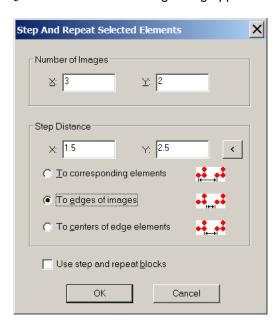
We have specified 3 copies in X and 2 in Y which will create a matrix of 3 X 2, so 6 copies. The step between copies can be specified in the three ways shown. "To edge of images" will create the specified spacing between images, so 1.5 inches in X and 2.6 inches in Y.
